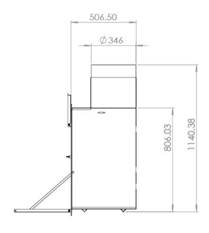
Surround is 25mm Wider than Unit All Round Braai Body Thickness = 2mm Braai Doors Thickness = 1.5mm Ember Maker Thickness = 3mm Surround Thickness = 4.5mm
