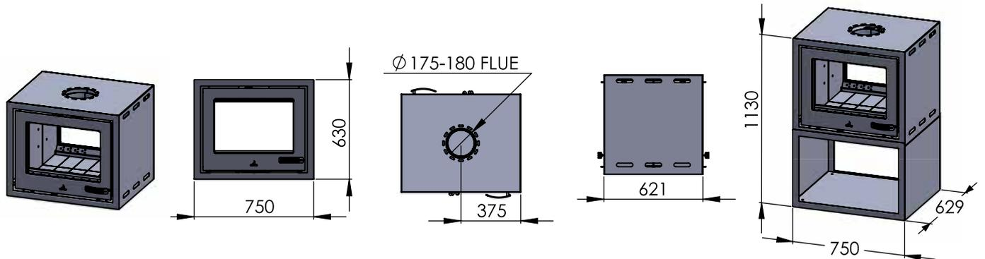
14Kw | Freestanding | Double Sided | Convection | 175 - 180mm Dia Flue | Top Exit Only
