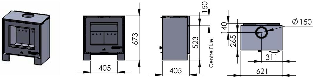
8Kw | Freestanding | Convection | 150mm Dia Flue | Top or Rear Exit
