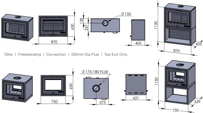
14Kw | Freestanding | Double Sided | Convection | 175 - 180mm Dia Flue | Top Exit Only
