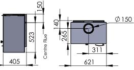
8Kw | Freestanding | Convection | 150mm Dia Flue | Top or Rear Exit
